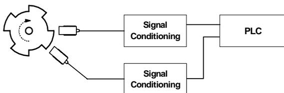
Figure 1: Simple speed measurement with checking.
