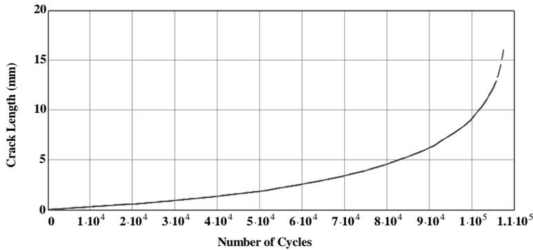
Figure 4: Crack growth rate against stress cycles.
