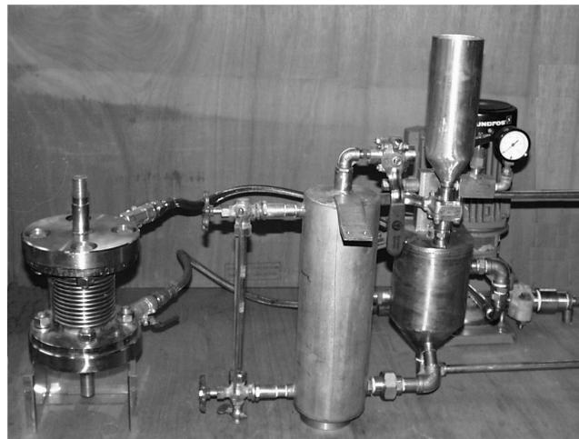
Figure 3: Fatigue test cell.
