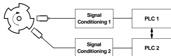
Figure 2: Modified speed measurement system with additional checking.
